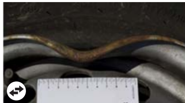
Wheel rim circumference, damaged non-compliant rim. Valuation of a dimensional check to check safe state of the vehicle
