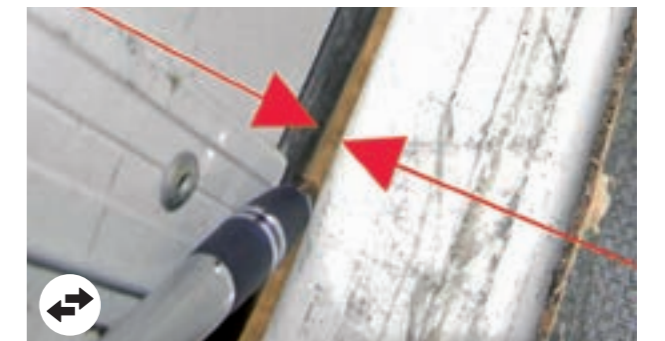
Deformations in the body closures not beyond economic repair, closure not possible or not sand-proof
