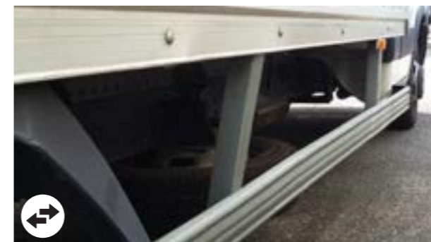
Side underun guards: Deformation within economic repair
