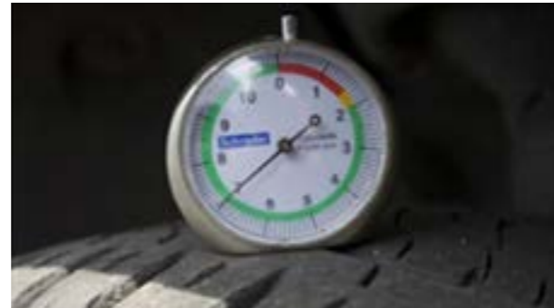
Tyres: Base of groove depth \geq 5 mm (CONFORMS) Note: The wear of the tyres is measured in the most worn groove on the tyre.
