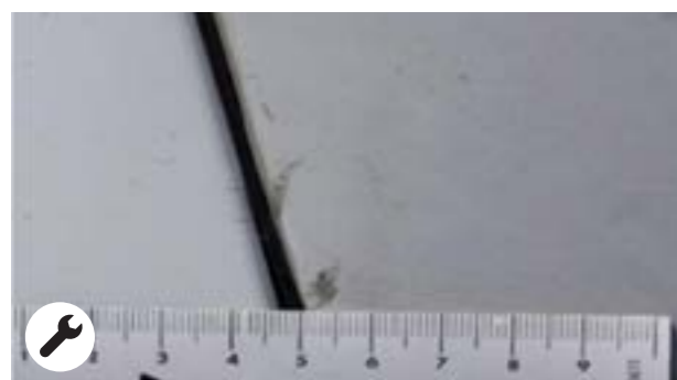
Difference in shade following repair NB: Tolerance accepted linked to ageing of the vehicle
