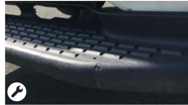
Rear footboards: Deformations within economic repair
