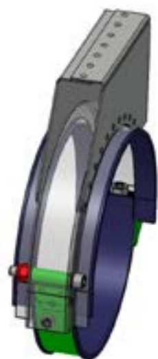
Band to tank bracket fastening: check the status of components (oxidation, fatigue, etc.)
