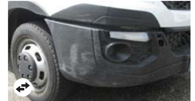
Removal of material or deformation feasible or economical to repair
