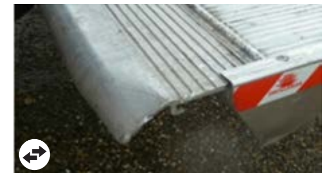
Tail lift: Deformations of platform within economic repair
