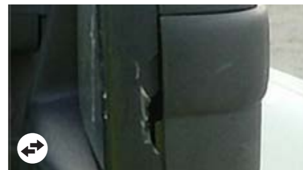
Removal of material, broken part
