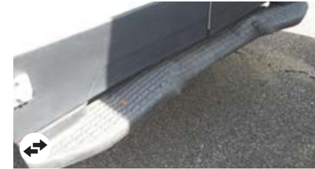
Rear footboards: Deformations not within economic repair
