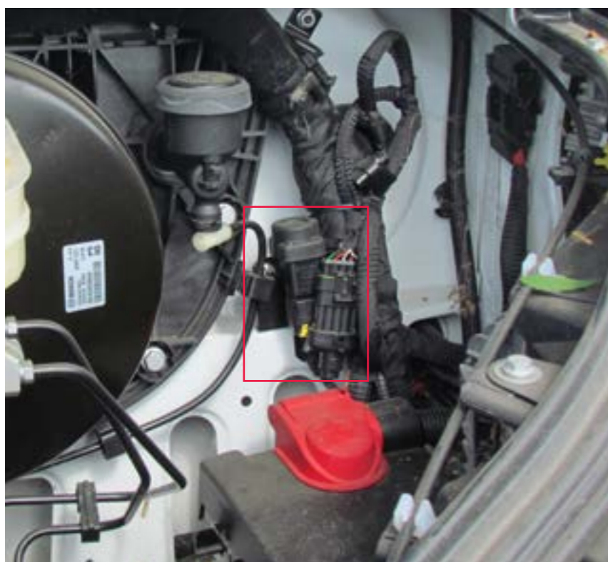
FIS: Inertial Safety Switch
