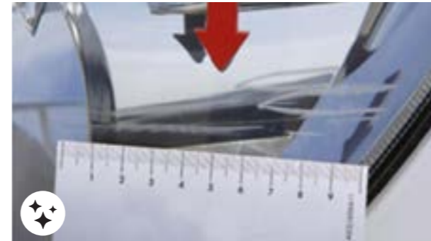
Deep scratch (with removal of material), outside of lighting field and sealed light
