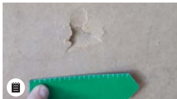
Wood internal protections: Small impacts
