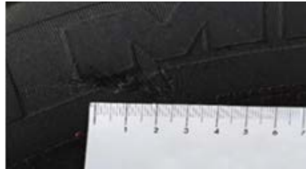
Tyres: Notch \leq 3 mm deep (CONFORMS)
