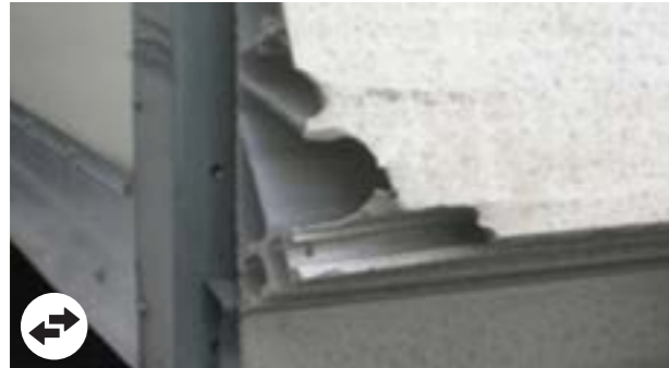
Tail lift: Deformations of platform beyond economic repair, broken or incomplete trim
