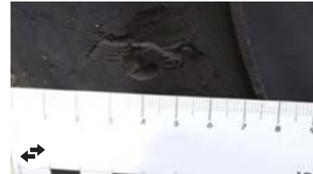
Tyres: Notch > 3 mm deep, removal
