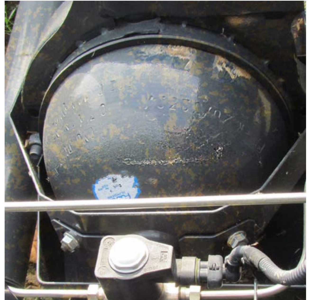
Original CNG cylinder identification markings absent or illegible
