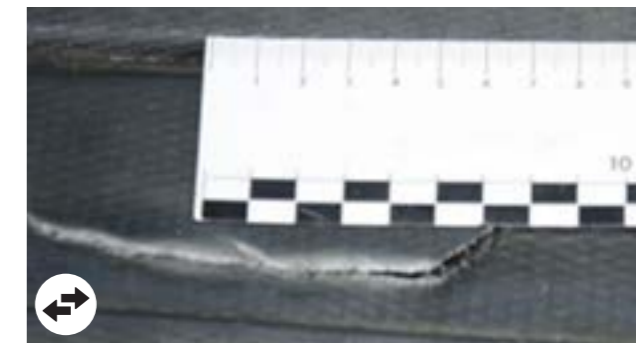
Perforation of hard plastic trims. Repair of hard plastic trims 1 hour flat rate if aesthetically acceptable and repairable
