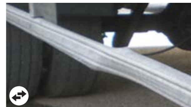
Side underun guards: Deformation beyond economic repair
