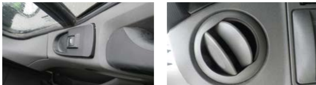
Slight discolouration due to sun exposure
