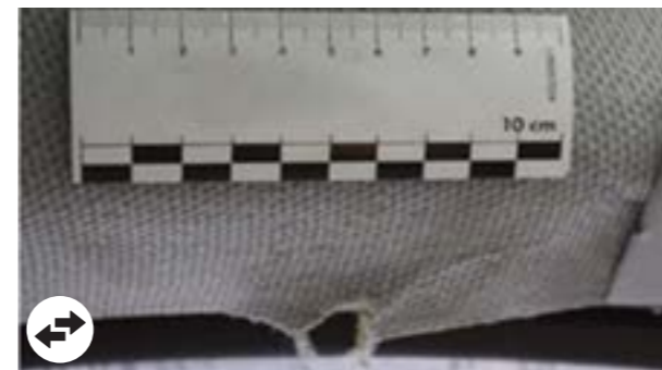
Fabric trim: Tear, hole > 5 mm, indelible marks
