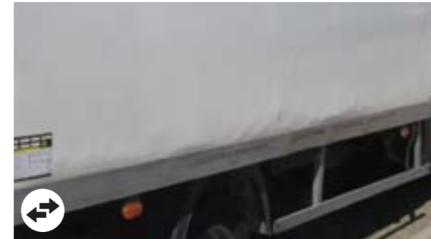
Fibreglas side panels: Deformation on lower part, length of > 1 m NB: Replacement of the front panel of the underbody requires removal of the underbody.
