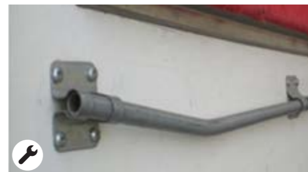
Upholstery and rods: Rods and upholstery deformed within economic repair
