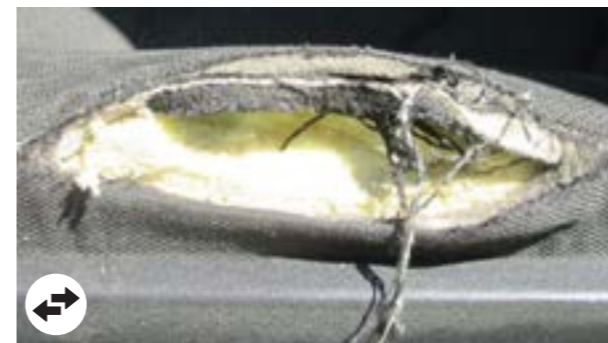
Foam missing or broken frame
