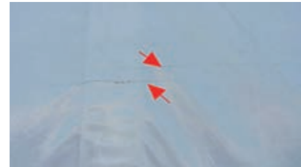
Deep scratches through to the fabric
