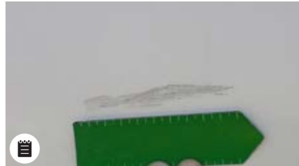
Side panels: Faint scratch with material removal ≤ 10 cm
