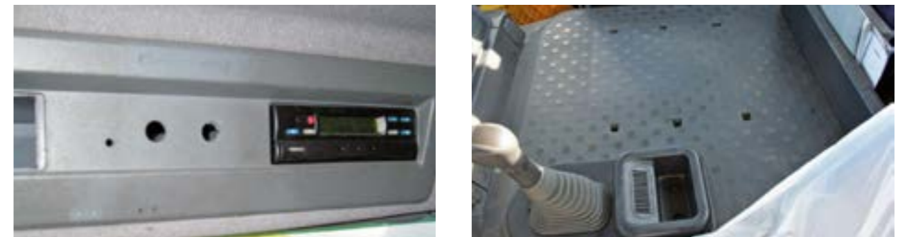
Control parts, seat or trim pieces missing, broken or pierced
