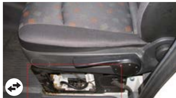
Missing equipment or trims
